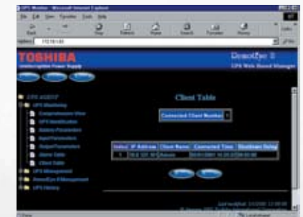
RemotEye II's web interface allows a user to view the protected machines RemotEye II oversees.
